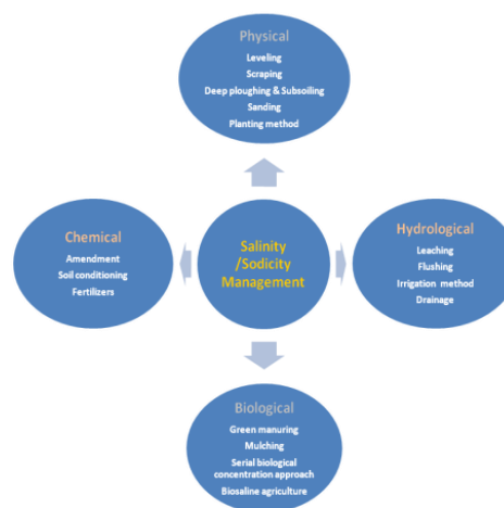
FIGURE 3 Integrated soil reclamation approach
