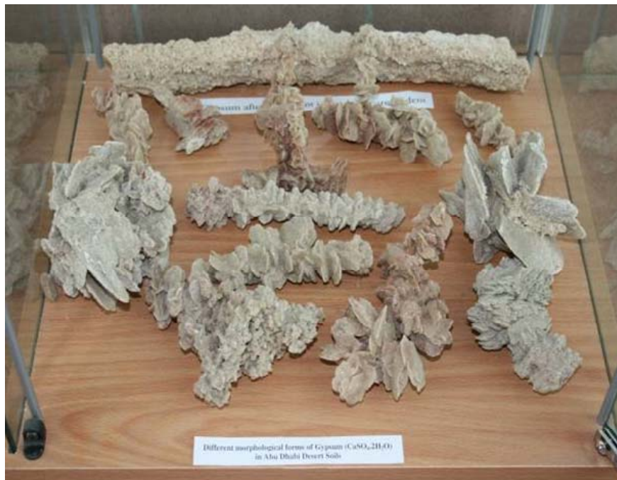
Rough surface tubular form (rear) along with serrated type elongated gypsum form (center)
