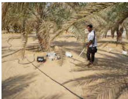
■ Figure 6. The light stick being used to measure the light interception fraction ( LI ) of the cultivar ‘Shahlah’ under the high salinity treatment S3 (15 dS m -1 ). The light stick is 1 m long and comprises 20 equi-spaced quantum sensors that record photosynthetically active radiation at 2 Hz.
