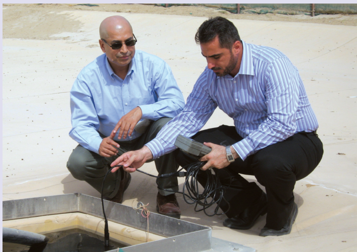
Evaluating water salinity in the low saline tank at ICBA – a key parameter for measuring water quality.
