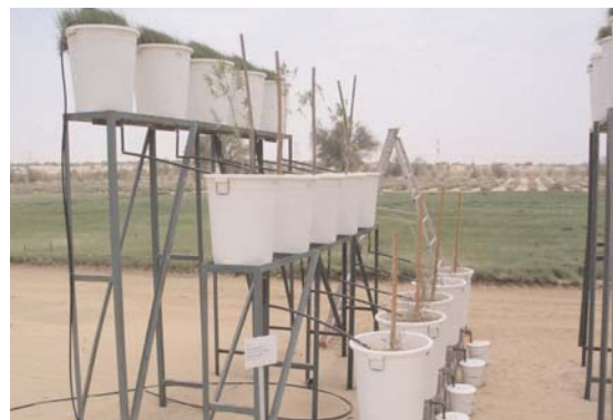
Experiment to determine drainage water use and salt balance of grass and shrub species in the three-step lysimeter
